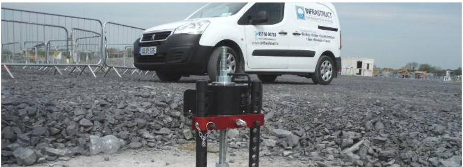
Proof Load Testing to 140kN
